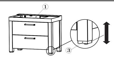
Per una corretta installazione controllare con la livella ① la "messa in BOLLA" In order to install the product properly, please check its leveling by using the spirit level
